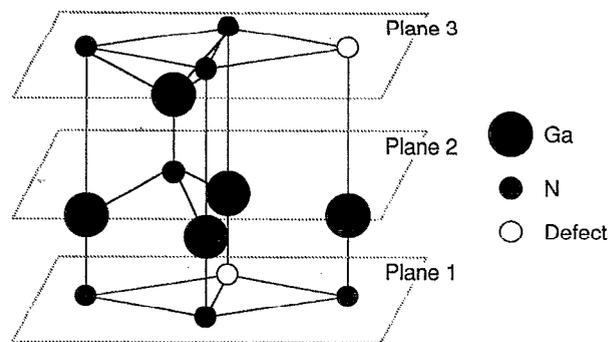
FIG. 4. A primitive wurtzite-structure  $\alpha$ -GaN unit cell in which one N atom is replaced by a vacancy.
