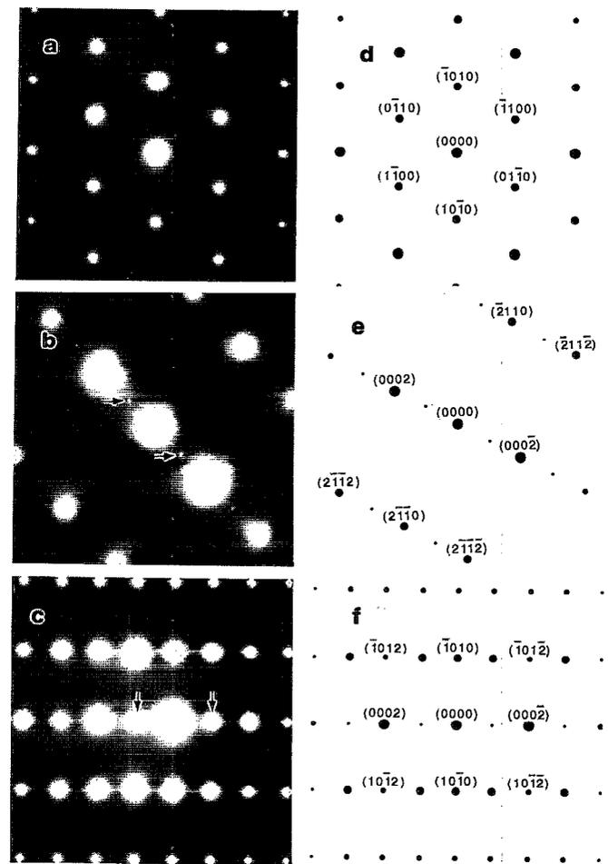
FIG. 2. Experimental and simulated zone-axis electron-diffraction patterns from GSMBE  $\alpha$ -GaN. The zone axes are (a) and (d) [0001], (b) and (e) [01 $\bar{1}$ 0], and (c) and (f) [ $\bar{1}2\bar{1}$ 0], respectively.
