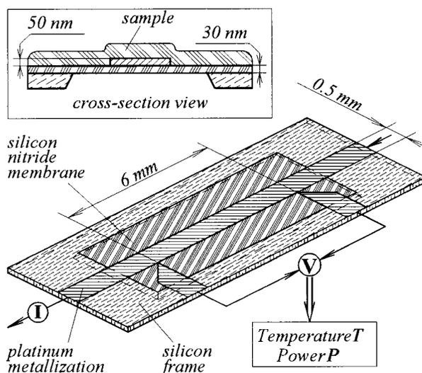
**Figure 1.** MEMS-based calorimetric sensor for TDSC (not to scale).
